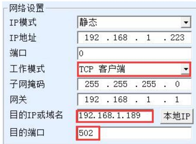
picture10 Modbus TCPBe a client.
