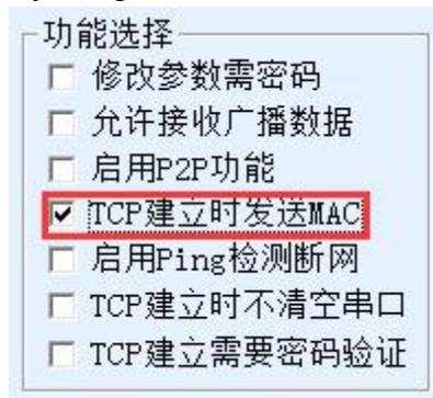
picture31Send on connectionMACAddress
