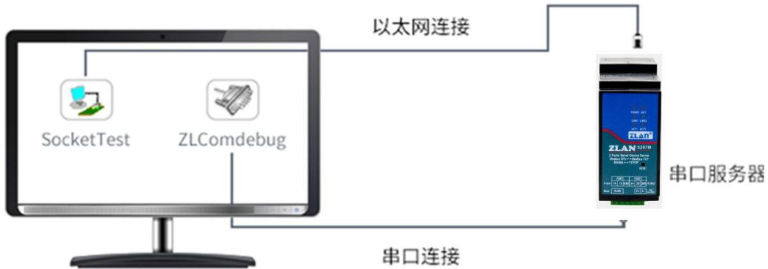
picture9 TCP Communication diagram
