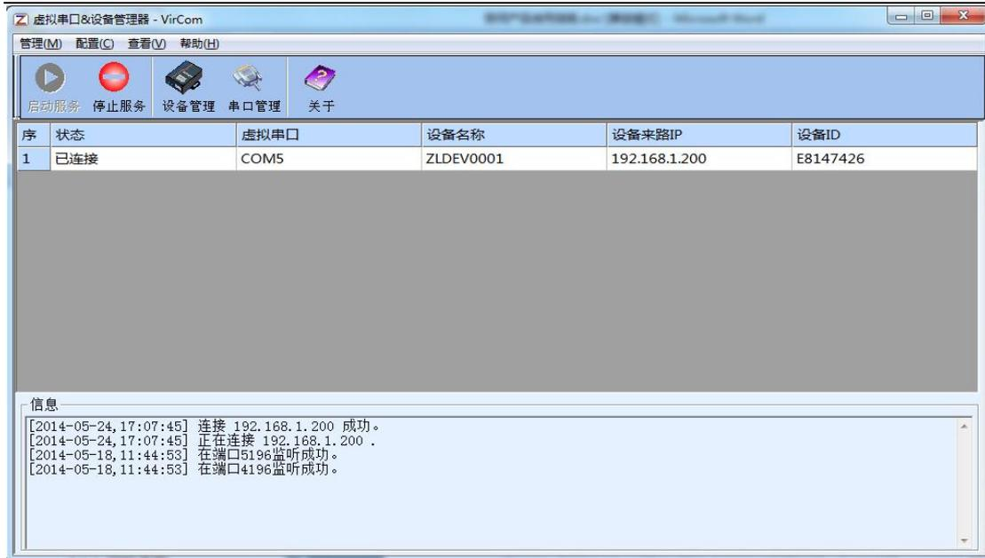
picture7The virtual serial port has been connected
