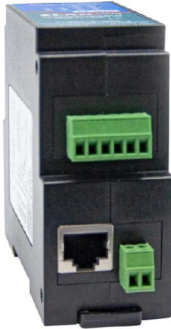
picture4Power supply, network port, serial port1、 Serial port2
