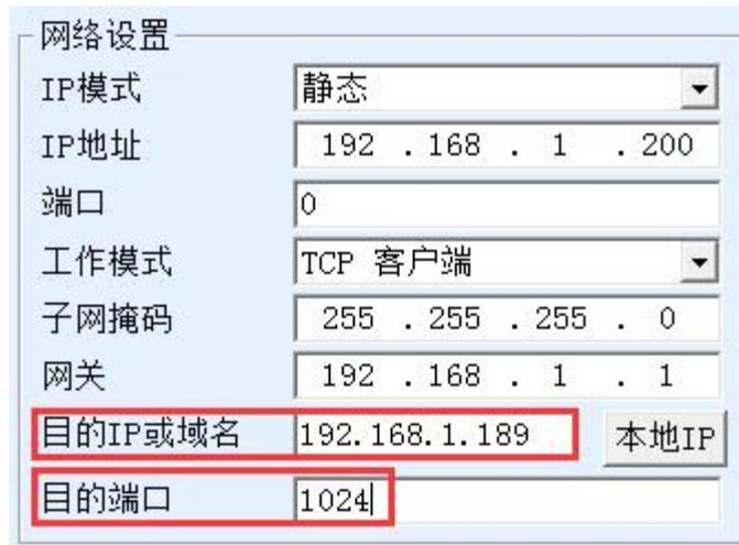
picture14The first purpose IP and Port
